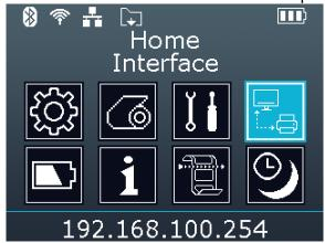
WLAN Factory reset is available in Interface > WLAN > WLAN Factory Reset When the printer is turned off, the wireless LAN setting is applied as the factory default
