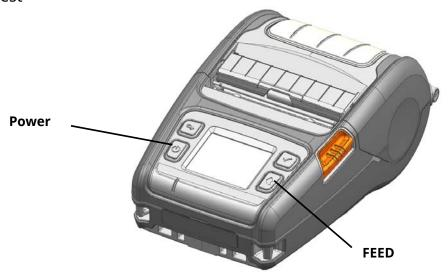
While the printer is turned off, turn on the printer while pressing the feed button. The printer setting values will then be printed.
